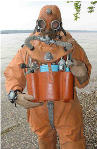
This is a Russian IDA-59, a fully closed circuit re-breather. The original purpose of the device is to be a submarine bailout apparatus. Maximum operation depth is 300m (1000ft) according to the original manual.
